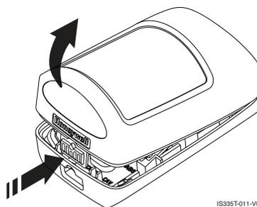
1. Press firmly on housing latch.
