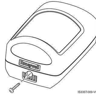
1. Close the sensor and apply power to the sensor. Initialization is complete when the LED stops flashing slowly (less than 45 seconds).
