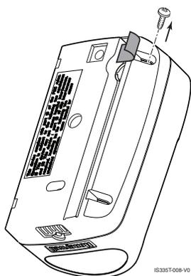
Remove tape from back housing and retrieve cover locking screw.
